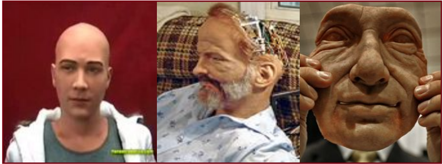
Each Hanson robot emerges as a four-dimensional sculpture. The presence of character arises from the interaction of the mechanics, the Frubber, and the intelligent software, to affect any of 2 to the power of 361 possible expressions
