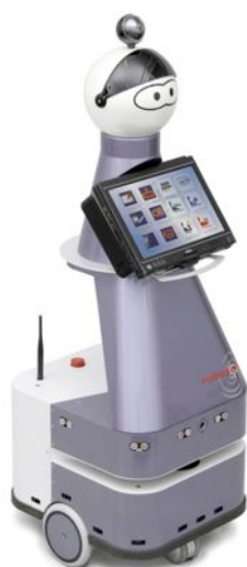
Kompaï has been designed to assist dependent persons at home. This robot can speak, understand what is said to it, find its way around the house and, with just a word, access internet services.
